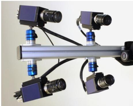
The AutoGrid® product family enables for strain analysis on samples and components in sheet metal industry. It proved well suited for a variety of applications in deep drawing and hydroforming as well as for different materials including aluminium alloys, stainless steel, and fibre reinforced composites.
