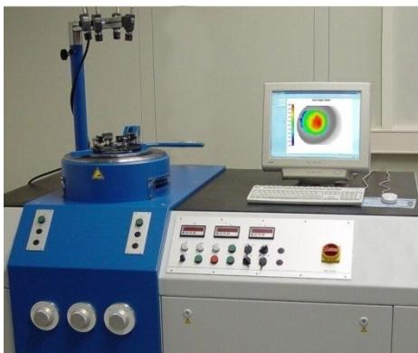
The AutoGrid® *in-process* has been designed to meet our customers' needs for flexibility in the optical set-up, measurement volume and local resolution. The direct, fast and accurate measurement is based upon the automatic evaluation of grid patterns that are either printed or electrochemically etched. The system is able to determine a field of strain values up to more than 100 % without any unambiguity.
